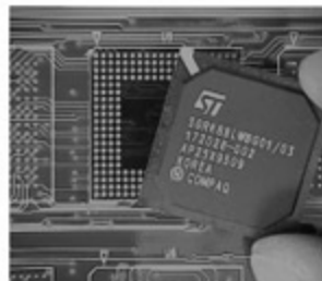
11. Gently place the properly conditioned part aligning the balls or leads of the part with the filled apertures.
