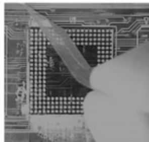
9. Remove the masking tape applied to the periphery of the reworked area applied in step #7.
