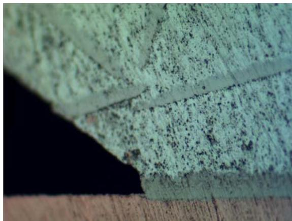
**Figure 3- Microstructure of BGA/pad interface at 500X**
