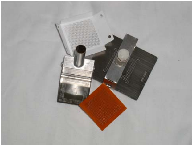
Figure 2. Various types of stencils.
