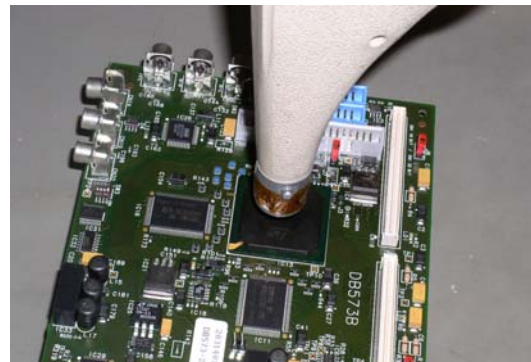
Figure 11. Hot air gun being used to solder a BGA.
