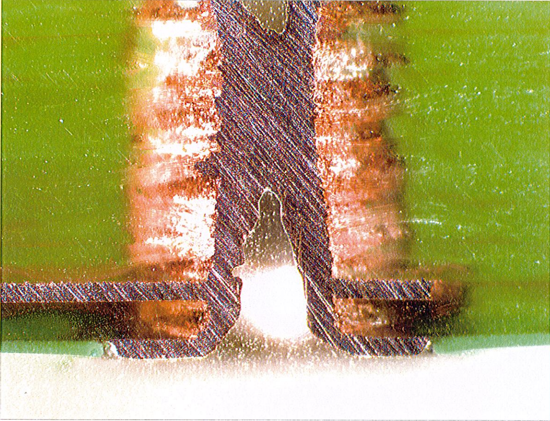
Illustration 4: S/N TB833036 50X magnification. Inner layer connection looks good.
