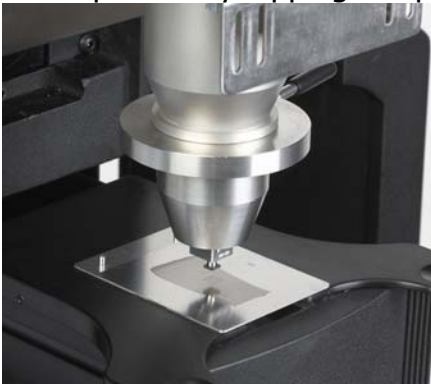
Figure 2 Flux Dipping of BGA (OK International Inc.)
