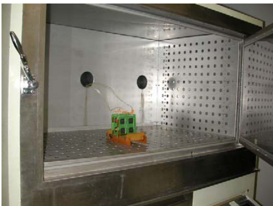
Figure 7- Test boards in Thermal Cycle Chamber
