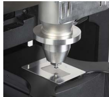
Figure 5 Flux Dipping of BGA (OK International Inc.)
