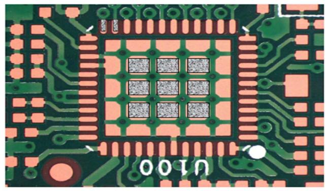
By placing soldermask plugs in the thermal vents on the ground plan and then putting strips over the plugs and creating a windowpane area for soldermask which create less flux and more open space for the solder to lift the part up. Only place solder paste in the marked areas to reduce the flux but it will still give you similar and effective thermal dissipation. Then place solderpaste on the pads.
